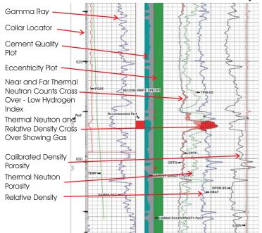
**Shallow Gas** - The cased hole analysis tool shows formation gas as per the thermal neutron density cross over (shaded in red). The near and far thermal neutron counts are also scaled to suggest zones with low hydrogen index (low porosity or gas). The casing cement plot estimates the amount of bulk material just behind casing and the eccentricity plot estimates the casing to formation centralization. Both are used to create a calibrated formation density
