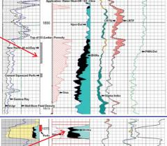
Original completions began to water out. Evaluation of reservoir fluids identified water "fingering in" across upper reservoir
