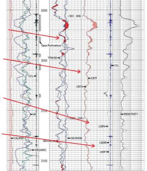
N2 Flood Showing Break Through - In a N2 injection field, intervals of break through were identified by comparing the open hole data to the Cased Hole Analysis tool data set. The data showed an increase in gas (N2) saturation across the upper three intervals
