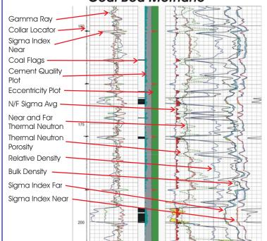
**CBM** - The processed thermal neutron, epithermal neutron and formation density data from the cased hole analysis tool, identifies coal and grades potential of each using various inputs (i.e. bulk density, gamma ray, neutron and density porosity, etc...). Each coal is analyzed individually with a report summary generated in addition to log type products.
