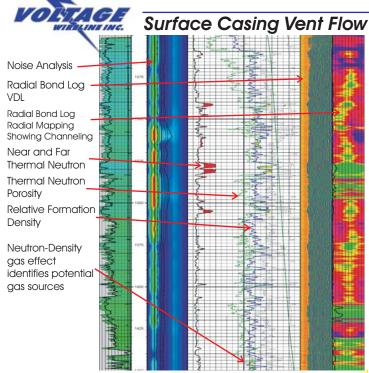
**Surface Casing Vent Flow/Gas Migration** - Gas flowing outside the pipe may be identified by a Noise Temperature survey. Cement bond quality may be evaluated with the aid of a Radial Bond Log. The Cased Hole Analysis Tool is used with these services to build a "story" of what is actually happening. The Cased Hole Analysis Tool pinpoints the formation gas source causing the problem while identifying annular gas completing the picture.
